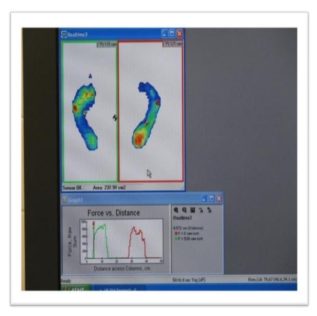
The *F-Scan*® measurement system is used in gait analysis and research on the effectiveness of interventions.
